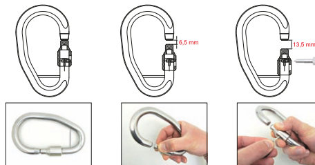
REST POSITION closed gate MANUAL OPENING for passing through the plates EMERGENCY OPENING WITH KEY for evacuation from safety line
